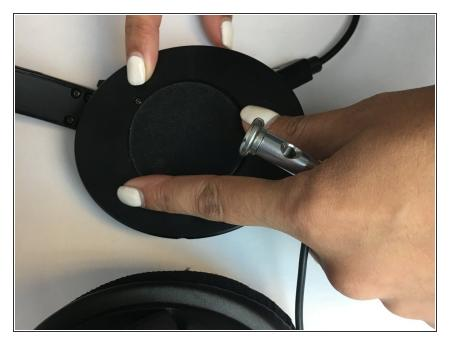
• Unscrew the 1.10 screws with T3 size screws that hold the front plate.
