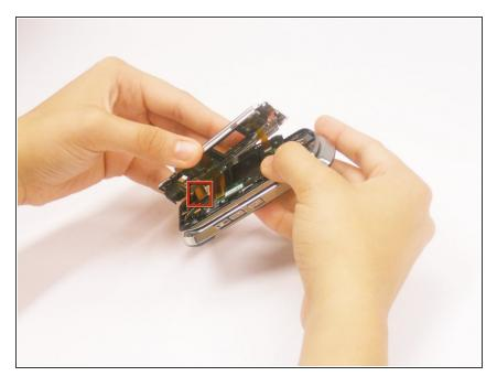
Use the flat end of the plastic opening tool to unclip the cable ribbon from the logic board
