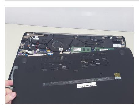
Carefully remove the back panel to reveal the inner components.
