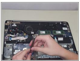
Using the JIS screwdriver along with the J000 head, unscrew the four Phillips PM2.5x5.5 screws, and place them aside.
