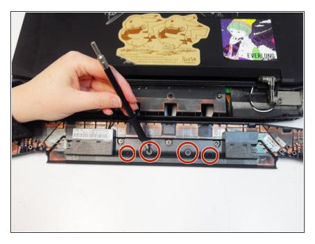
The speaker is attached to the hinge cover by four 3.5mm Phillips #00 screws. Unscrew and remove them.
