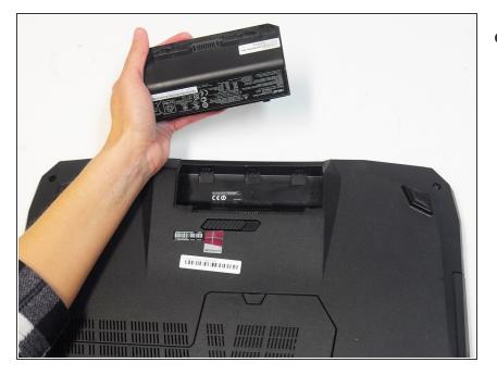
Remove the battery from its compartment.
