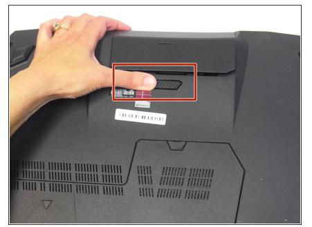
Slide the battery release latch all the way to the right. This will cause the battery to "pop" out slightly.
