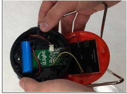
After the lens has been removed the back cover needs to be removed. There are no snaps or screws holding it in place.
