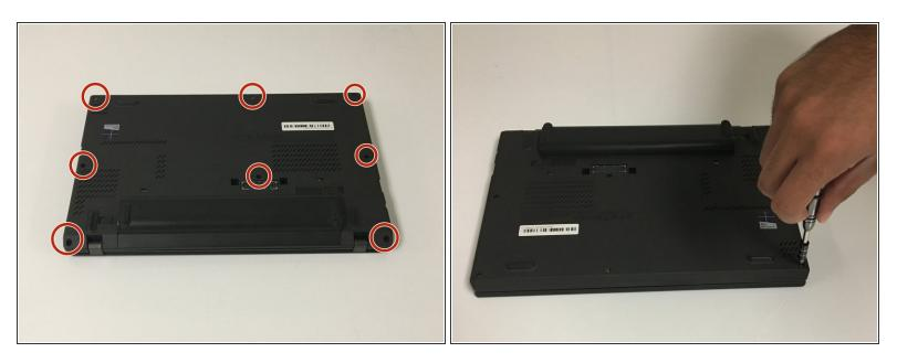
Remove the 8 0.2mm Phillips screws connecting the back cover to the laptop.
