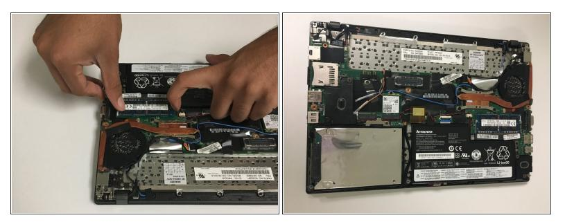
• Remove the RAM stick by carefully popping its holders out of place.
