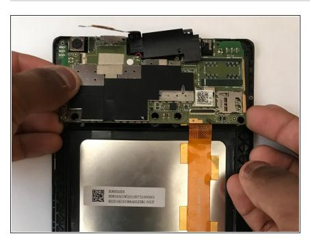
Lift up the motherboard carefully, ensuring that you lift the speaker housing and the motherboard together
