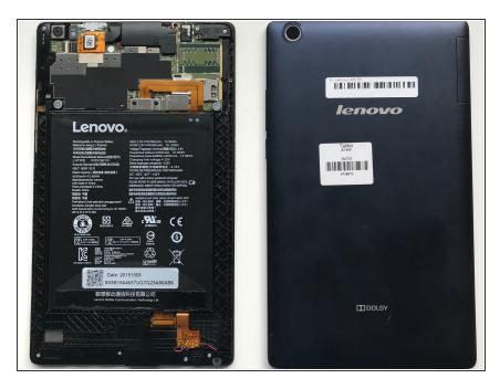
• Remove the back cover by prying it open with the metal spudger tool.
