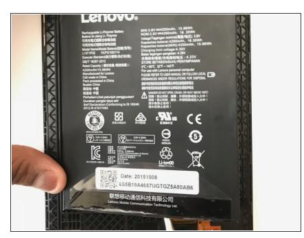
• Remove the battery by lifting it up using a plastic spudger.
