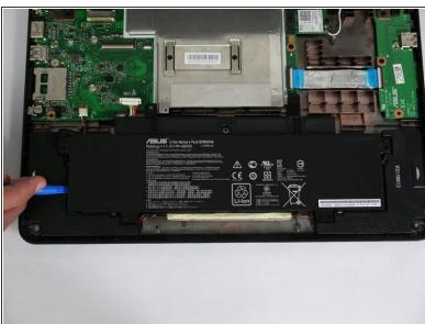
At this point, using the plastic removal tool, lift the battery out of the shell.
