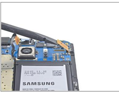
Using the flat end of a spudger, disconnect the touchscreen connector.
