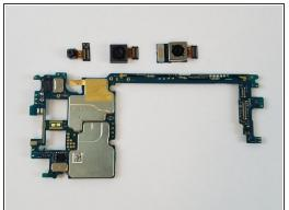
• Remove the two rear-facing and front-facing cameras from the motherboard.
