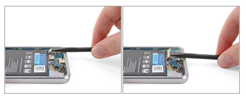
Use the flat end of the spudger to lift up the two press connectors on the bottom end of the motherboard above the USB-C port.
