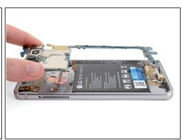
Grab the motherboard by the top end (the end with the cameras) and gently lift it up and out of the phone.
