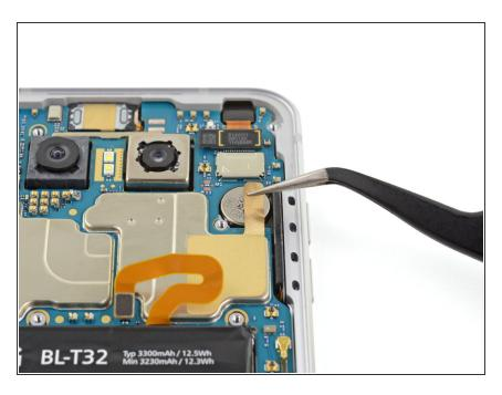
Remove the sticker connecting the motherboard to the vibration motor.
