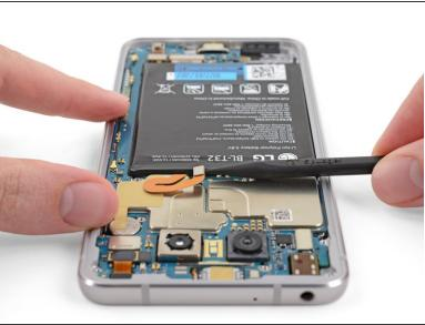
Use a spudger to pry up the press connector at the end of the battery's ribbon cable, disconnecting the battery.
