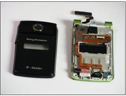
Use a plastic opening tool in the indicated location and apply pressure until the case hook is detached. Then lift the case up until the two pieces are detached.
