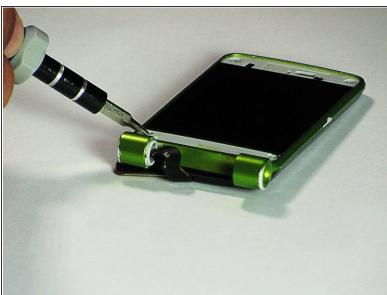
Remove the four 5.4 mm screws with a Torx T5 screwdriver.
