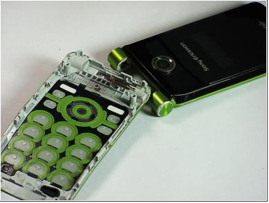
Separate the bottom and top half of the phone from the hinge they are connected by.
