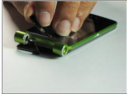
The top and bottom covers are held in place by adhesive. To remove them, use a pushpin in the four indentations indicated to remove.
