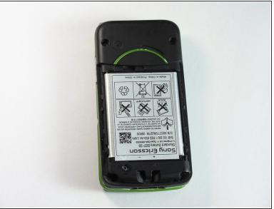
Remove the two rubber casings for the top two screws with a plastic opening tool.
