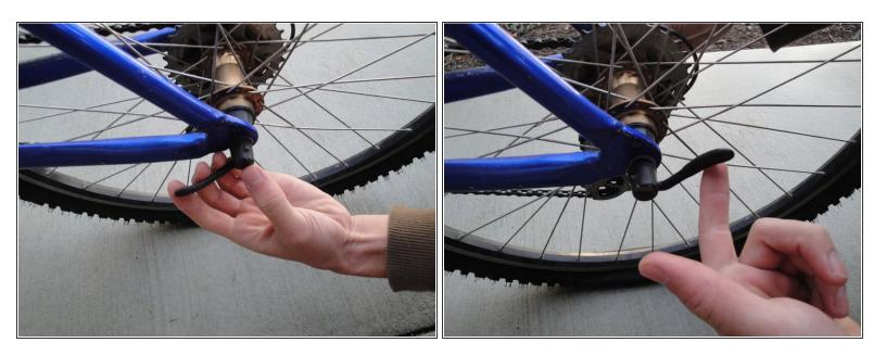
Flip the quick release lever on the wheel.
