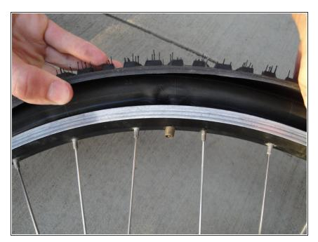
Remove the tube by pushing the valve through the hole in the rim and pulling the tube out from under the tire.
