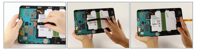
Lift the retaining tab and withdraw the black LCD ribbon.
