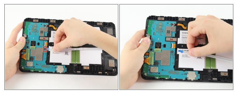
• Remove the adhesive film, lift the retaining tab and withdraw the white speaker ribbon.
