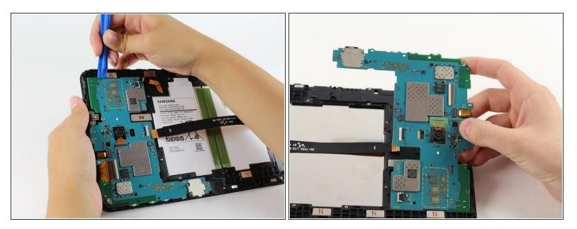
• Lodge the plastic opening tool under and lift the motherboard out of the tablet.
