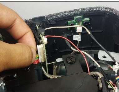
Remove the two cables connecting the motherboard to the front I/O panel.
