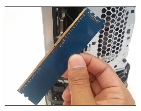
You can now easily pull the RAM out of the socket, and replace up to two new ones!
