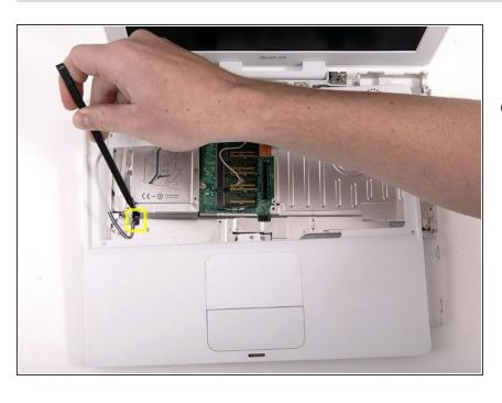
Lift the upper case off completely and disconnect the multicolored speaker cable from the logic board.
