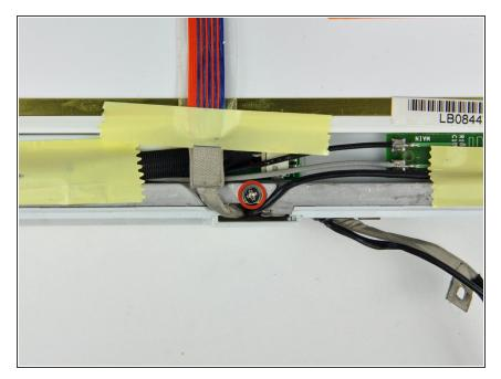
Remove the second of the two Phillips screws securing the clutch cover to the cast aluminum frame of the clutch hinges.
