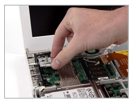
Lift the modem and modem shield from the bottom.
