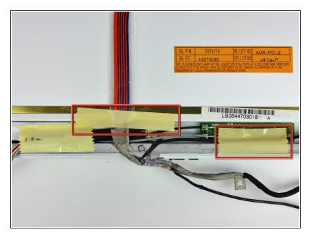
Remove the two pieces of tape over the display data/microphone cables near the lower edge of the display.
