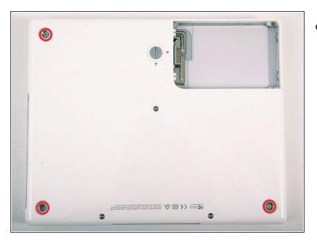
Remove the three newly-revealed Phillips screws.
