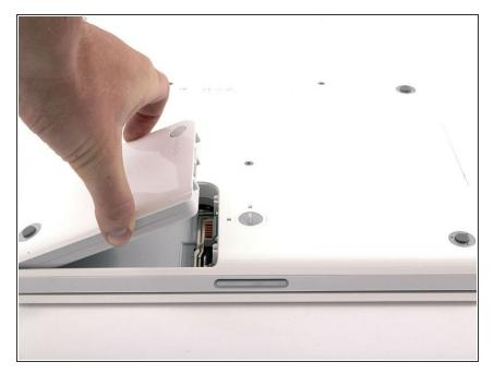
Lift the battery out of the computer.
