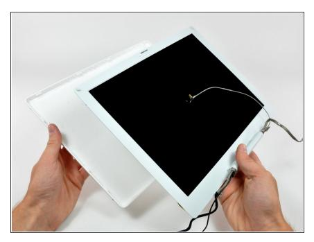
Lift the rear bezel off the display.
