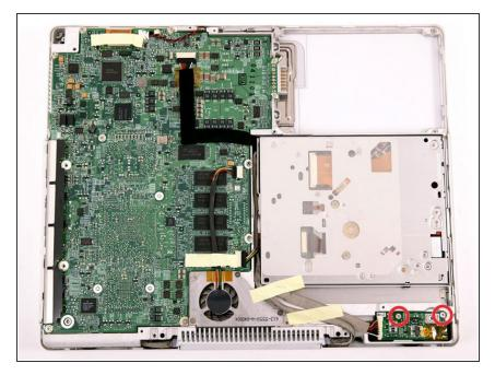
Remove the two Phillips screws securing the DC-In board.
