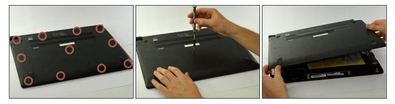
• Turn laptop over and unscrew the eleven M2 x 6.0mm back cover screws with the Phillips #0 screwdriver.
