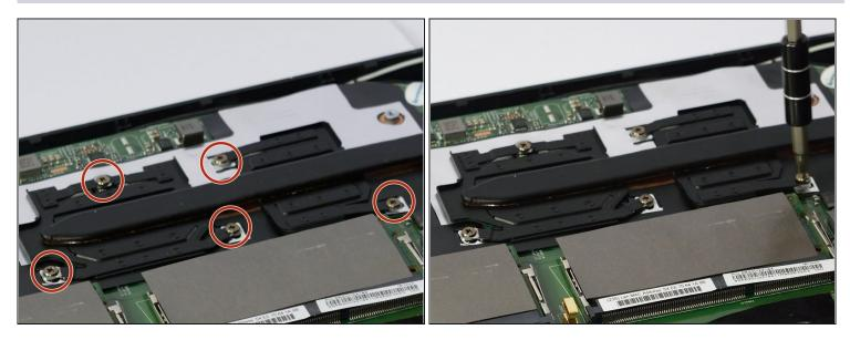
• Remove the five M2 x 4.0 mm screws from the heat sink with a Phillips #0 screwdriver.
