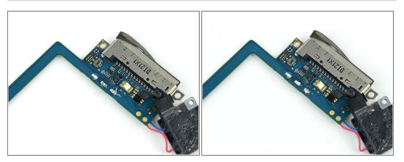
Next, use the tip of a soldering iron to flatten out the solder on the logic board solder pads. The
