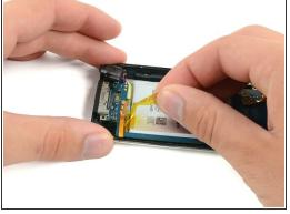
if necessary, use a plastic opening tool to peel the piece of yellow kapton tape located near the bottom of the battery.
