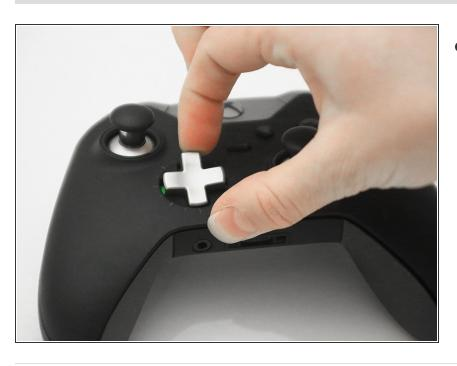
Remove the cross D-pad by pulling up on the top of the cross.
