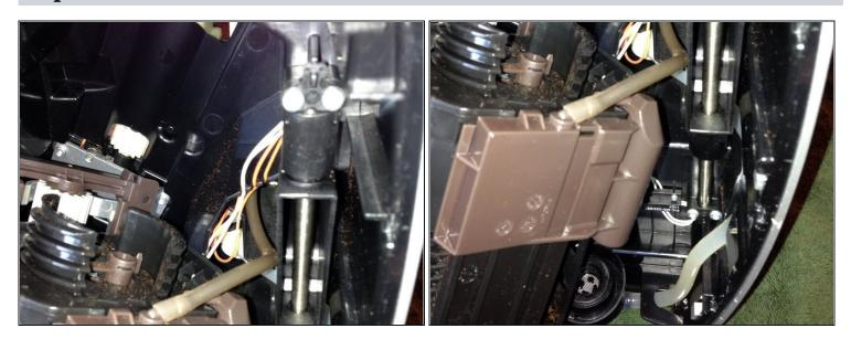
• Tamper Assembly Removed - Top
