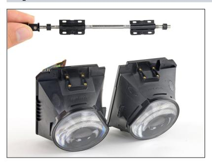
Remove the focus rod and its brackets.
