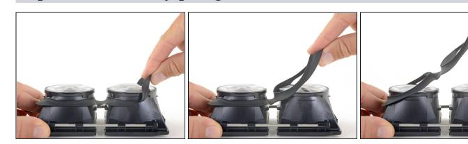
Gently lift the eyepiece gasket off of the lens and OLED frames to remove it.
