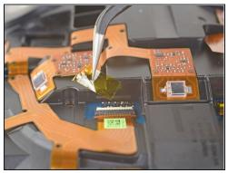
Use tweezers to remove the clear tape over all four of the sensor array cable connectors.
