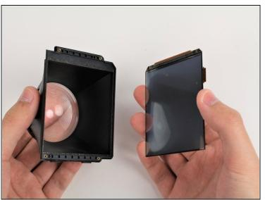
Remove the screen from the eyepiece housing by pulling the two pieces away from each other.
