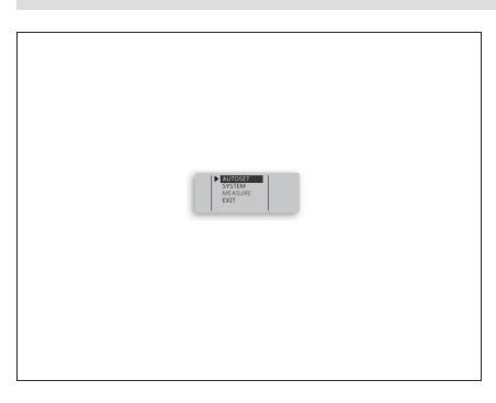
When you are finished measuring, make sure to reset the offset and custom settings by selecting the menu, then pressing AUTOSET.
