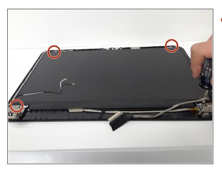
Remove the 4 M2 X 3mm Philips LCD screws.
