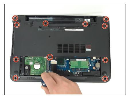
Remove 12 M2.5 X 5MM Phillips bottom palm rest screws.
