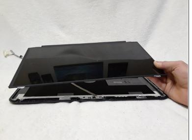
Unplug the screen cable and remove the screen.
