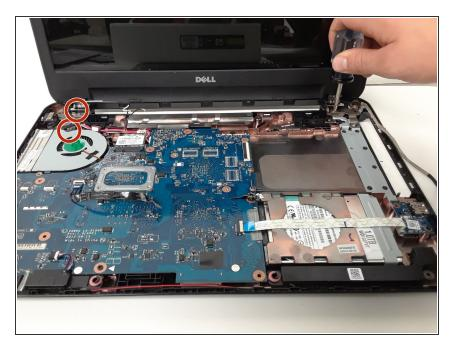
Remove the 1 M2.5 x 5mm Phillips left hinge screw and 2 M2.5 x 5mm Phillips right hinge screw.
