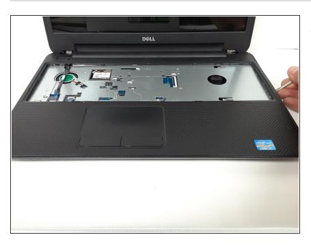
Use a small flat screwdriver to pry the palm-rest off of the computer.
