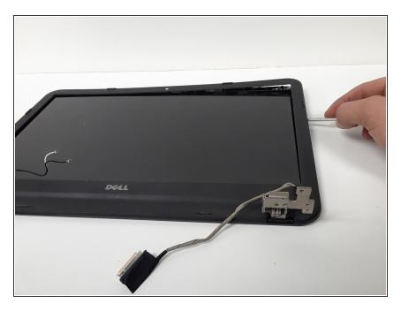
Pry off the LCD bevel using a small flat screwdriver.
