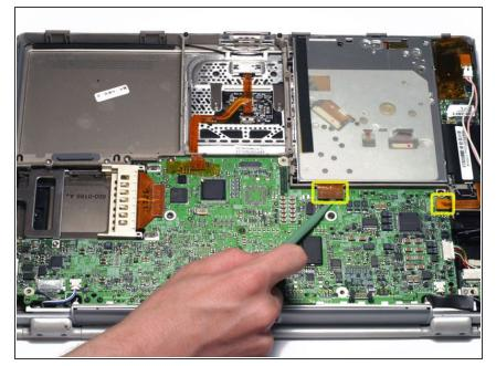
Disconnect the two orange connectors from the logic board, removing tape as necessary.
