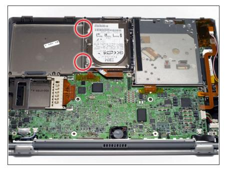
To free the hard drive, remove the two T8 Torx screws from the right wall of the battery housing.
