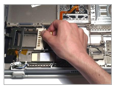
Remove the PC Card cage by pulling it to the right and twisting slightly toward you.
