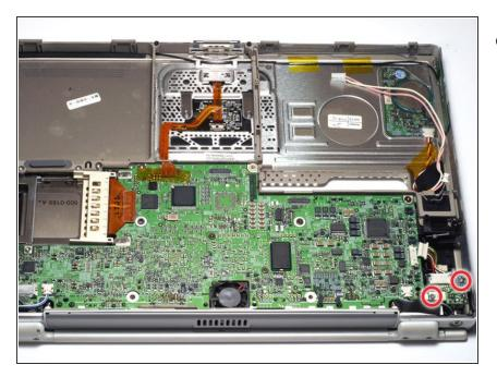
Remove the two T6 Torx screws from the DC-In board.
