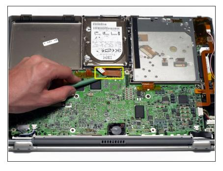
Disconnect the hard drive ribbon from the logic board using a spudger or the tip of your finger.
