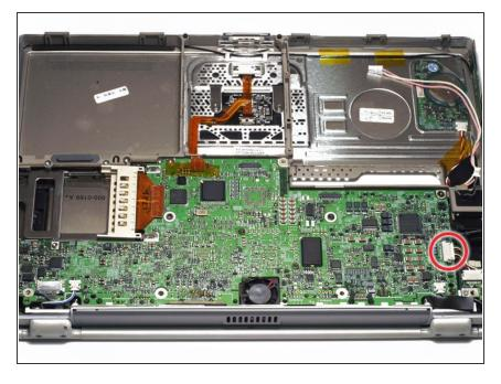
Disconnect the large DC-In connector from the right side of the logic board.
