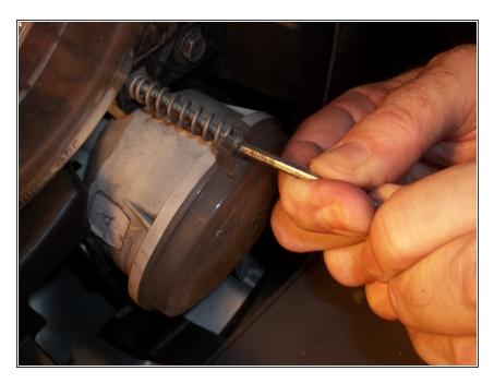
Using an allen wrench, turn the tension screw counter-clockwise to loosen the light housing.
