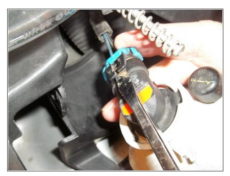
Remove the wiring harness from the light socket by lifting up on the tab with a flat-head screwdriver.
