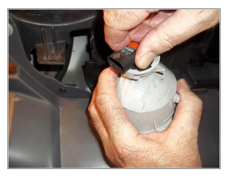
Remove the light socket from the light housing by turning counterclockwise.
