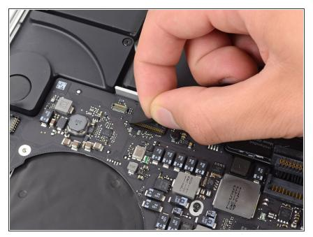
• Peel back any tape covering the keyboard ribbon cable connector.
