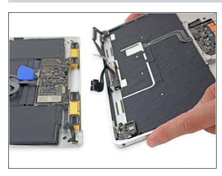
Separate the upper case assembly from the lower case assembly. To reassemble your device, follow these instructions in reverse order.
