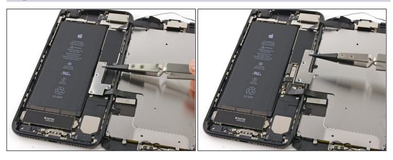
• Remove the lower display cable bracket.
