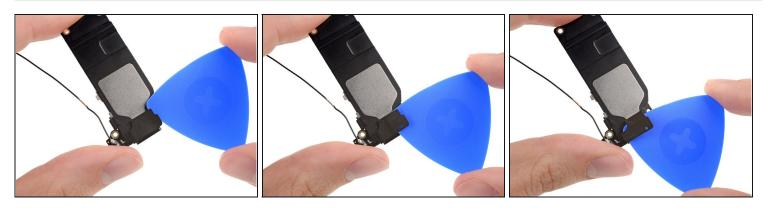
• Slide an opening pick between the antenna and the speaker on the right side, and carefully separate the adhesive underneath.
