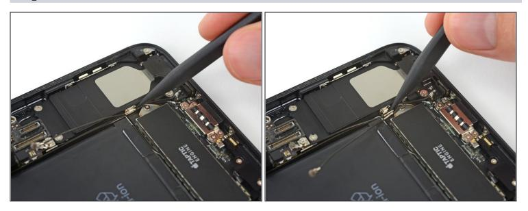
• Use tweezers or the point of your spudger to pry both coaxial cables out of the metal clip holding them on the side of the speaker.
