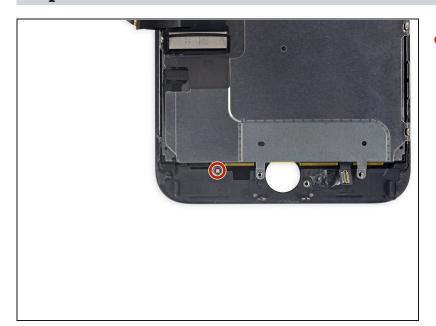
Remove the 1.8 mm Phillips screw securing the EMI shield near the bottom of the display.
