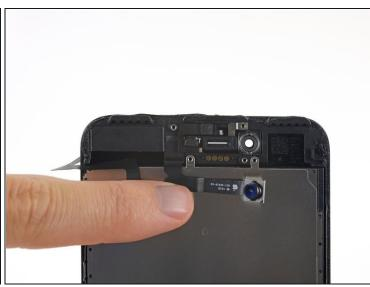
• Gently fold the camera and attached ribbon cable toward the bottom of the iPhone to allow access to the components underneath.
