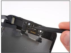
Slide the tip of a spudger underneath the proximity sensor flex cable, and lift the sensor out of its housing.
