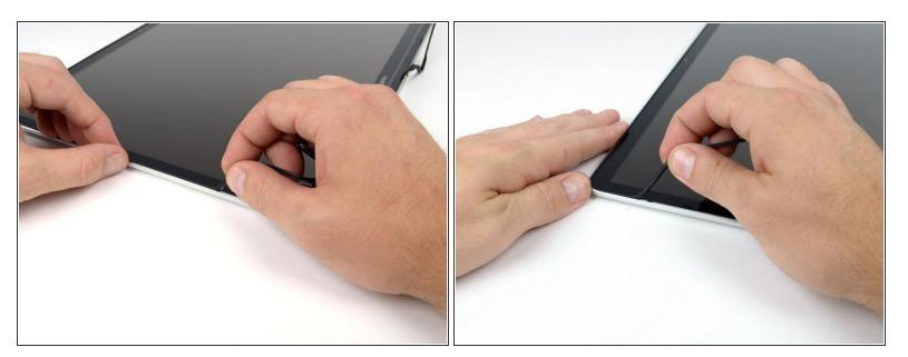
• Starting with the freed corner, pull the left gasket off the left side of the display assembly.
