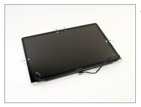
After prying up the three edges of the display glass, you should have four guitar picks resting underneath the panel, as shown.
