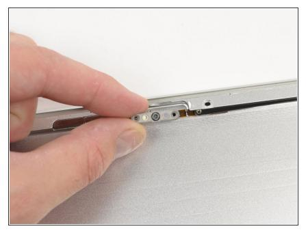
Lift and remove the camera assembly out of the rear display bezel.
