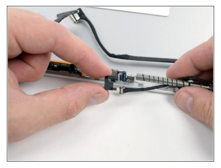
Once the cable is disconnected, remove the plastic bracket from the rear display bezel.
