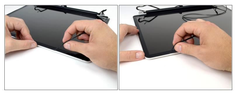
• Continue pulling the display gasket off the display assembly across the top edge.
