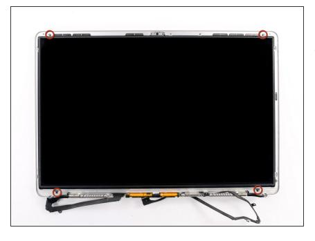
Remove the four 2.3 mm Phillips #00 screws securing the LCD to the rear display bezel.
