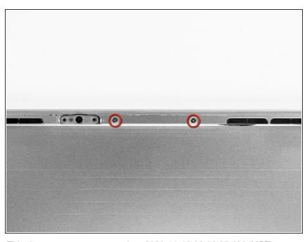
Remove the two 2.7 mm Phillips #00 screws securing the camera board to the rear display bezel.
