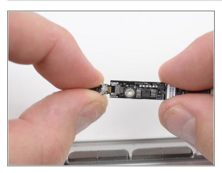
Pull the camera/AirPort cable straight out of its socket on the camera board.
