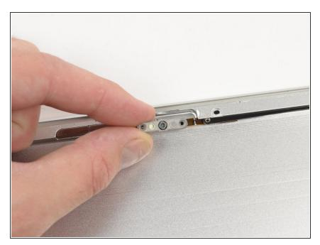
Lift and remove the camera assembly out of the rear display bezel.
