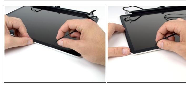
Continue pulling the display gasket off the display assembly across the top edge.
