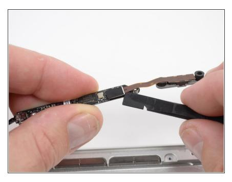
Use the flat end of a spudger to pry the camera board cable from its socket on the underside of the camera board.
