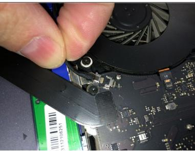
Pull the camera cable toward the optical drive opening to disconnect it from the logic board.
