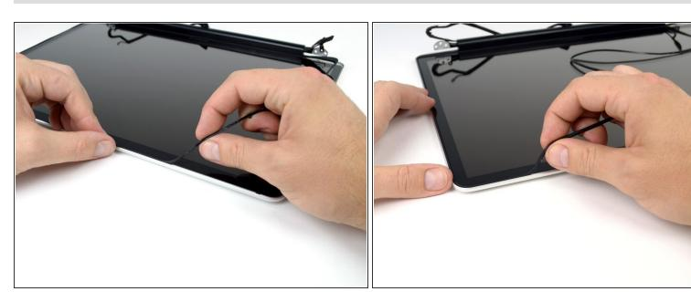
Continue pulling the display gasket off the display assembly across the top edge.
