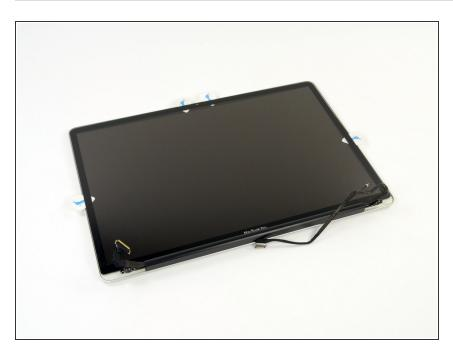
After prying up the three edges of the display glass, you should have four guitar picks resting underneath the panel, as shown.
