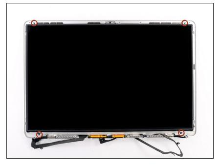
Remove the four 2.3 mm Phillips #00 screws securing the LCD to the rear display bezel.
