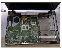
remove upper plate, revealing the main PCB.
