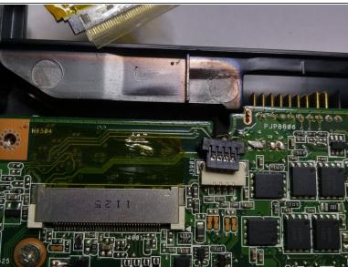
use IC extractor pliers to remove the cable away from is socket.
