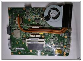
• lift the main board or motherboard up on the right side and slide it out.
