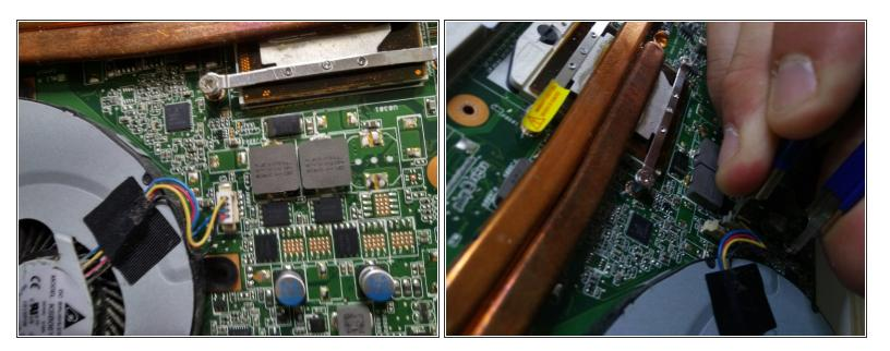
release the fan from the main board by removing the connector with an IC extractor pliers.
