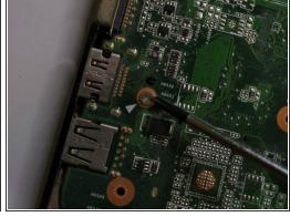
remove the 4 screws holding the main pcb ..
