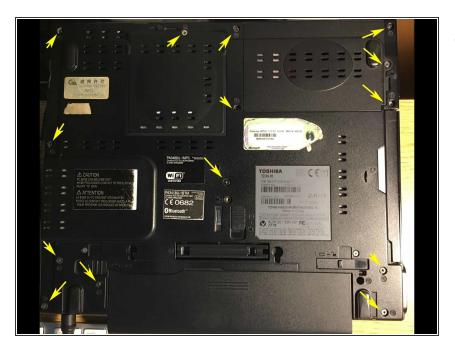
Power down the laptop. Flip it over and remove only the indicated screws.
