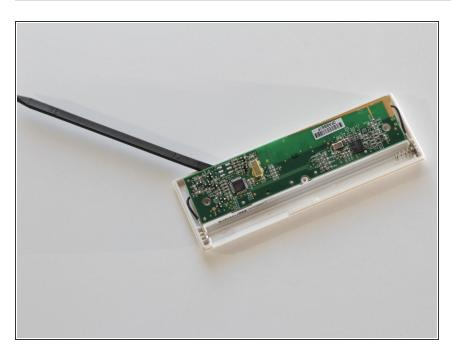
If your circuit board is stuck in the front panel, use a spudger to lift the circuit board from the front panel.
