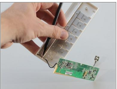
Using a spudger, gently pry the battery connectors from the front panel.
