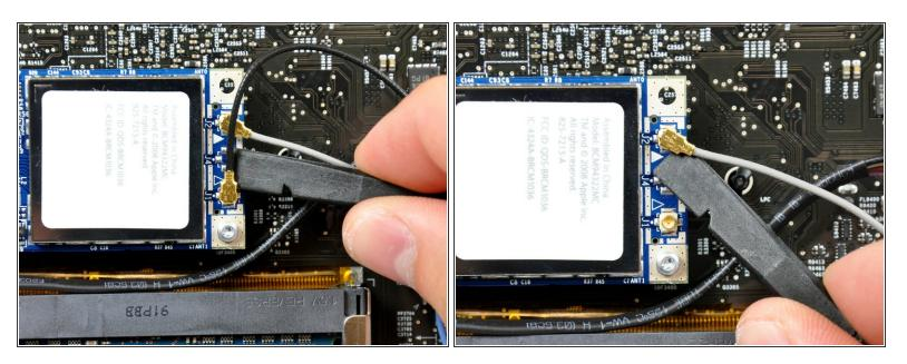
Use the flat end of a spudger to pry both antenna connectors up off the AirPort Extreme card.
