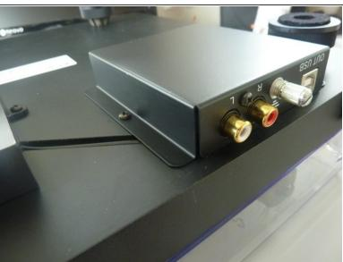
• Carefully turn the record player on its head. The preamplifier component is mounted on its bottom side. Unscrew the three philips screws of the metal casing, first the two screws that are fixing it to the wooden base plate, and then the third screw that is located between both RCA connectors.
