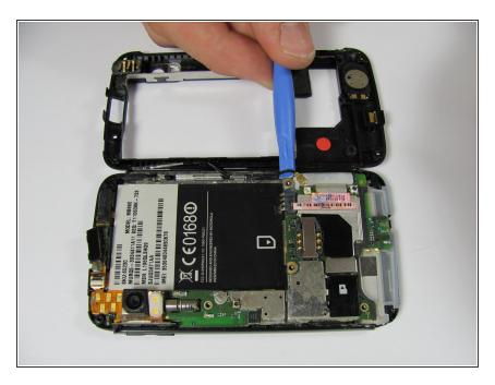
Disconnect the antenna from its housing on the motherboard by gently lifting beneath it.
