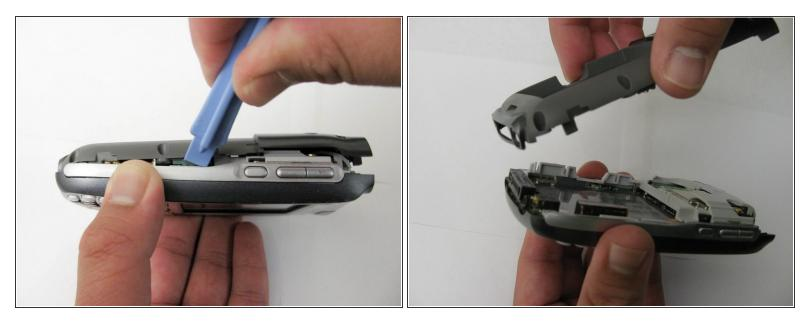
• Using the plastic opening tool, gently separate the back case from the phone body.
