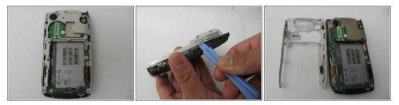
• Using a plastic opening tool, gently edge your way between the back and border case (Picture 2) until they are completely separated (Picture 3).
