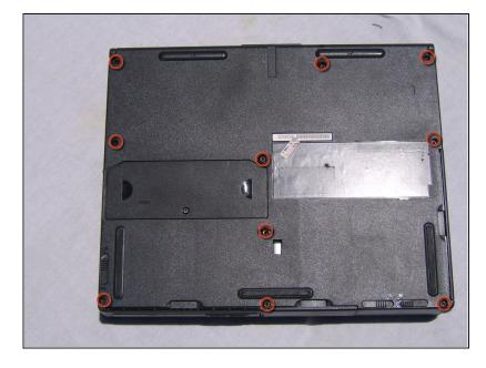
Locate and remove the 10 screws found on the bottom of the laptop using the <u>3.0 mm</u> <u>Flathead</u> Screwdriver.
