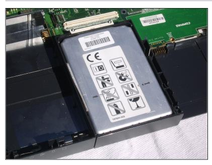
• Locate the HDD in the lower center of the laptop, found between the Battery and the Disk Drive.
