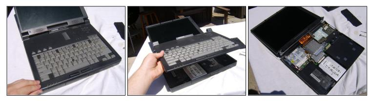
• Carefully lift the Keyboard free, raising it directly up and off of the laptop.
