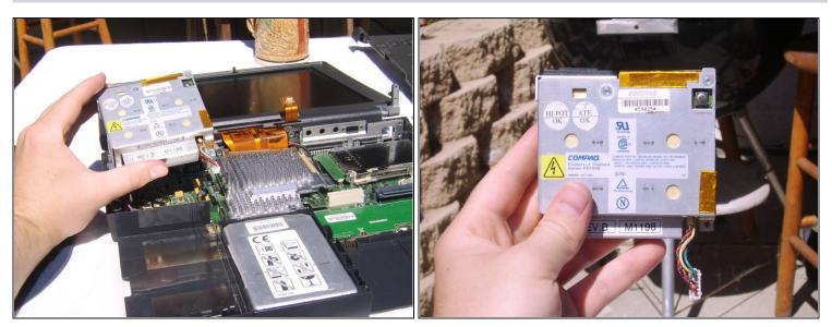
• Lift the Power Supply directly up and out of the laptop.
