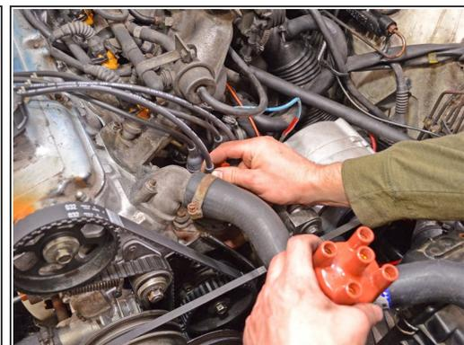
**i** Connect the spark plug wires to the new distributor cap one at a time. Mixing up the order will result in the engine not firing properly or at all.
