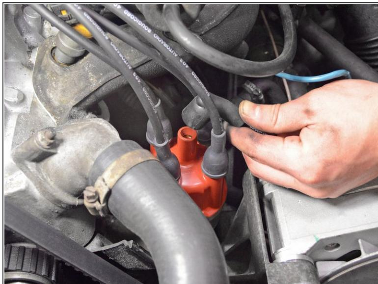
**i** The distributor cap is located next to the engine and has all of the spark plug wires connecting to it.
