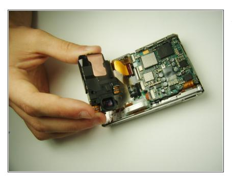
After releasing the clips, pull out black lens box.
