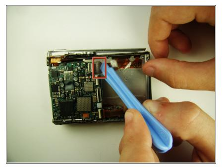
Use the plastic opening tool to flip the top clip that holds the ribbon to the motherboard unit.
