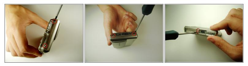
Locate and remove the 3mm screws on the top and sides of the camera with the size 00 screwdriver.
