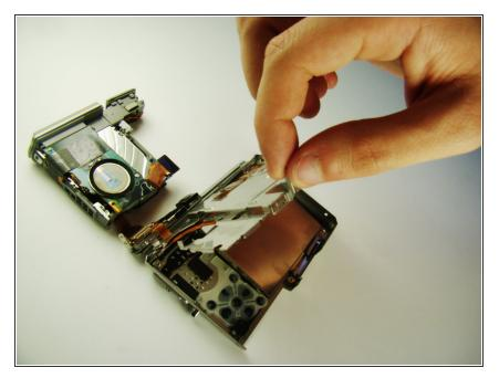
• Lift and remove the metal plate covering the LCD screen from the camera.
