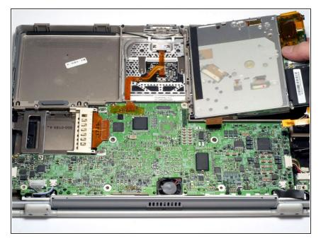
Remove the drive by lifting the right edge up and out of the computer.
