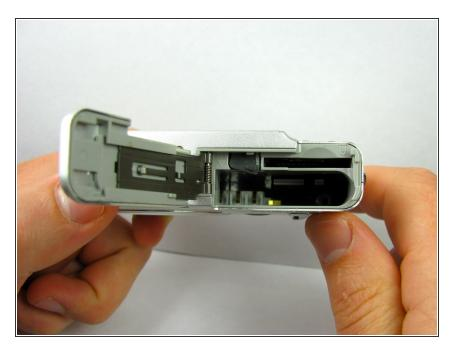
• The cover will spring open, revealing the battery compartment. Here is where you will remove or install the battery.
