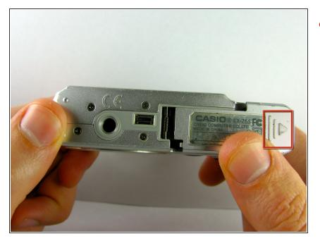
Slide battery compartment cover in the direction of the arrow located on the cover.
