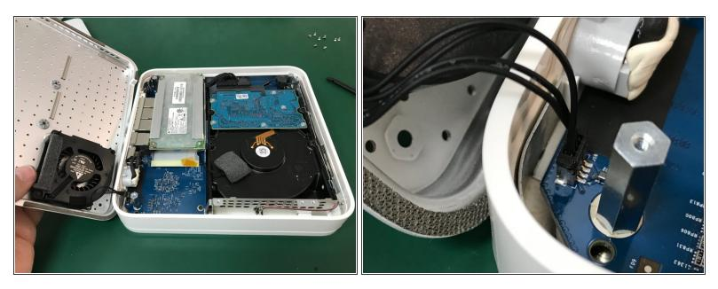
• With the tip of a spudger carefully remove the fan connector then remove the metal bottom cover.
