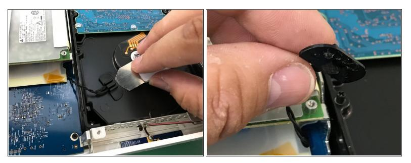
• Remove the clip that holds the temperature sensor and remove both.
