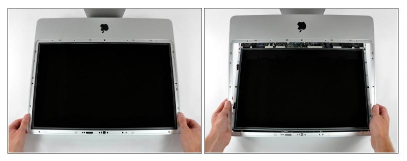
$\bigwedge$  The front bezel is still attached to the iMac by the microphone cable.
