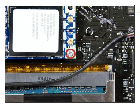
Remove the single T6 Torx screw securing the AirPort Extreme card to the logic board.
