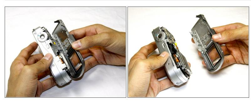
Once the screws are removed, slowly remove the back casing from the rest of the camera.
