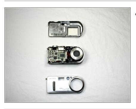
After the casing is removed, the camera should look as shown.
