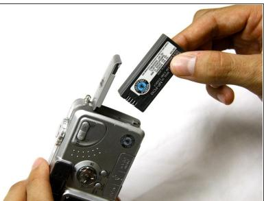
Remove the battery from the camera.
