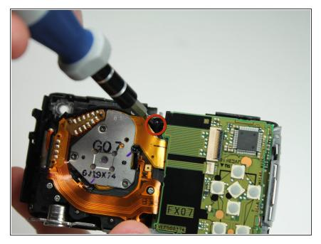
Remove the small screw in the hole towards the top of the camera(#00P, 5.4mm).
