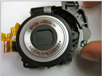
Now that the lens is fully exposed, remove the two phillips screws (4.34 mm) on front of the lens.
