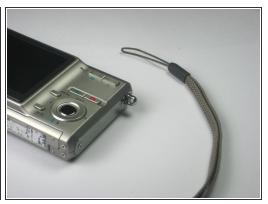
Remove the strap from the camera by pulling the thin cord out, creating a small loop, then pushing the thicker cord back through this loop.
