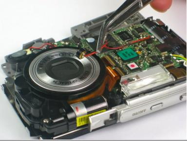
• Use a pair of tweezers to gently move the wire around part of the lens away from it so that you can access the lens.
