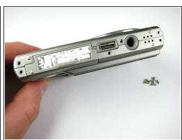
• Remove the six Phillips screws (3.69 mm) from the bottom of the camera casing.
