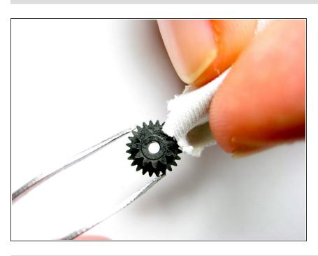
Clean the gear box and the gears with water and a cloth or paper towel. A pin can be useful to dislodge any grit or dirt stuck in between the teeth of the gears.
