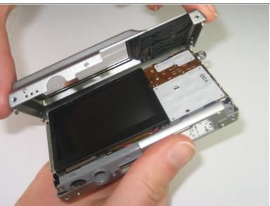
With the LCD screen facing up towards you, start at the bottom of the camera and gently pull off the back of the casing.
