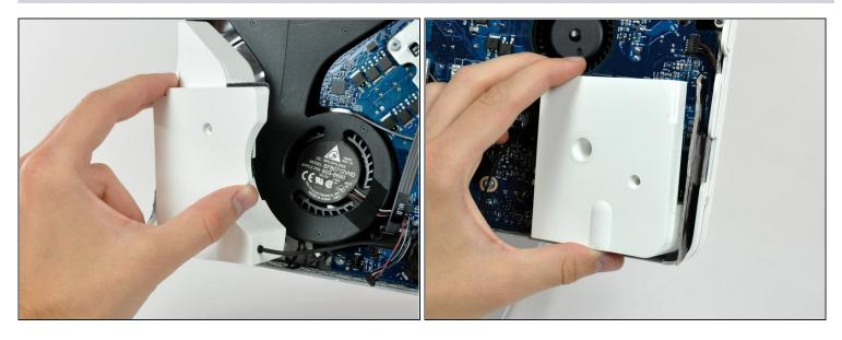
• Lift the left and right speakers out of the rear case.
