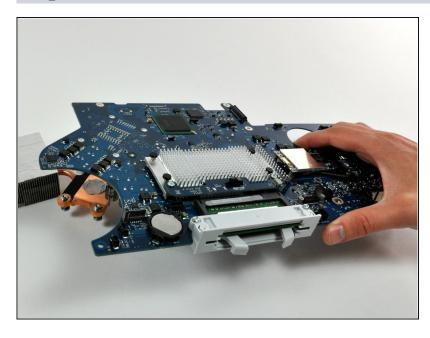
• Lift the logic board up off the heat sink.
