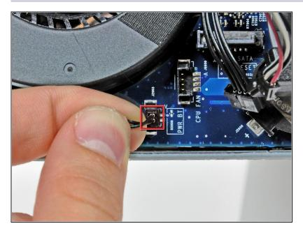
• Pull the power button cable connector up off its socket on the logic board.
