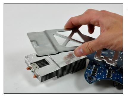
Lift the heat sink bracket up off the heat sink and the logic board.
