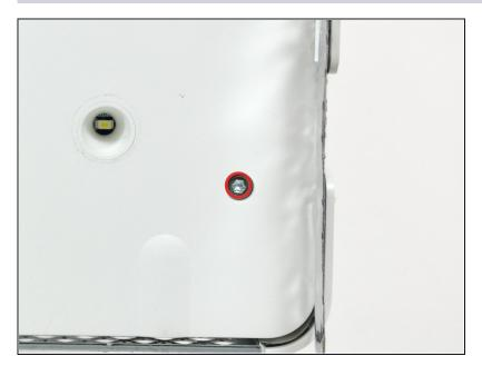
• Remove the 17 mm T10 Torx screw from the right speaker.
