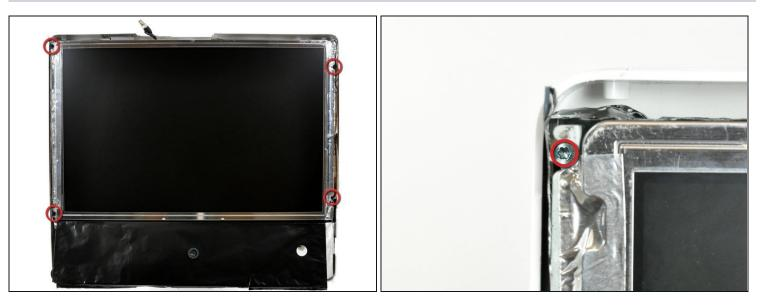
Allow the EMI shield to hang down from the display.
