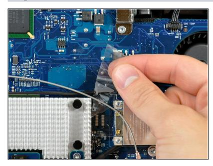
(i) If necessary, remove any tape covering the left speaker cable.
